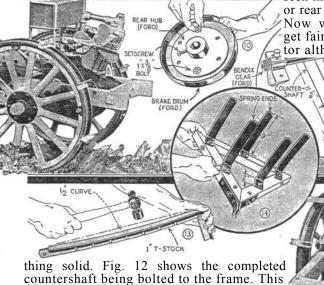
thing solid. Fig. 12 shows the completed countershaft being bolted to the frame. This must be done carefully, so that the bendix gear will mesh perfectly with the ring gear on the wheel. Test before going further by pushing the partly finished tractor backward and forward across the floor.
