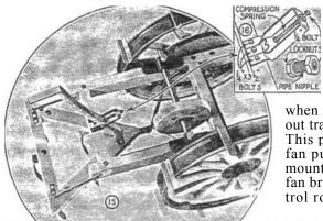
motor is mounted. Various engines will differ here, but in any case the metal support brackets should offer no difficulties. As there is no clutch on this tractor, it is evident that control must be through an idler pulley, which,
