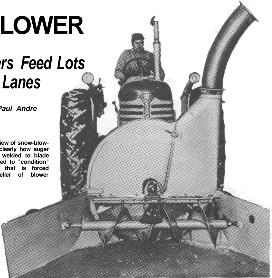
Forward end of auxiliary drive shaft is fitted with a universal joint that couples it to a system of chains and sprockets that drive blower impeller and a short jackshaft
