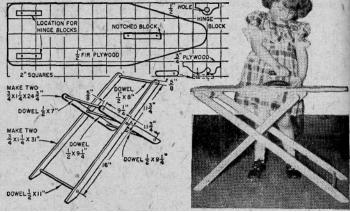
permits the board to be moved about without collapsing. Fasten the blocks with countersunk *fh* wood screws driven through from the top side of the ironing board. When assembling, the short-leg section must fit inside the long-leg section so the two will be flat against the board when folded for storage.—G. E. HENDRICKSON.
