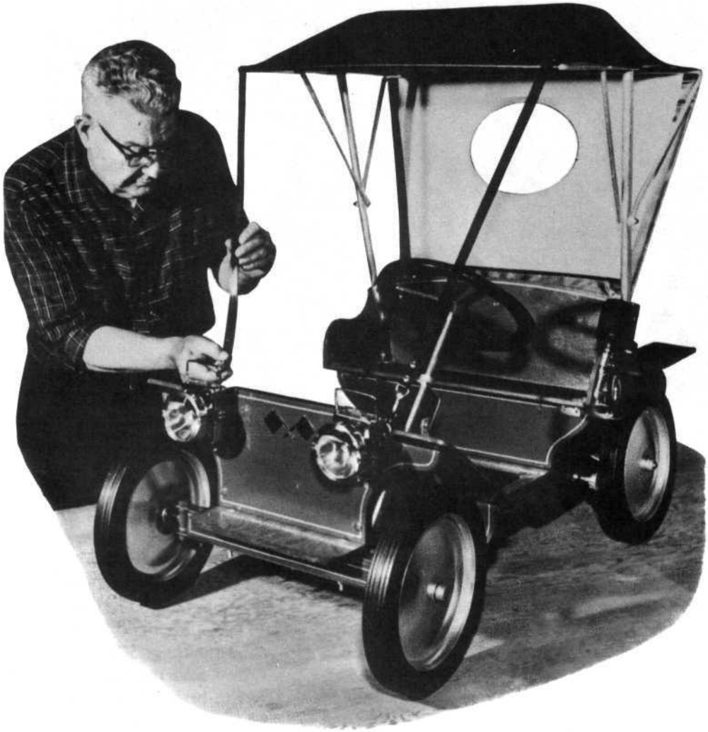
Swivel snaps riveted to the ends of straps hook into screweyes in the top edge of the dash
