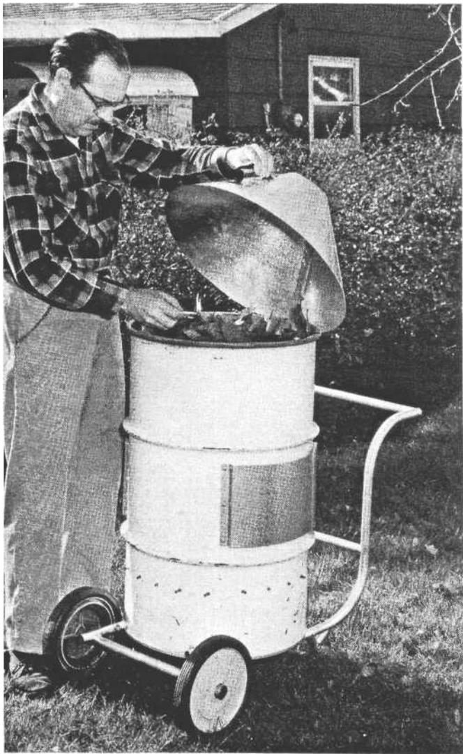
The burner may be used anywhere on your lawn without damaging the grass. When the 7-in. ash dump in the bottom is full, you merely wheel the cart to the trash heap and dump it with the flip of a lever
