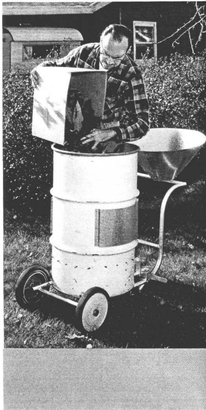
The 30-gal. steel drum is 31 in. high and has an inside diameter of 18 in., giving the burner a capacity of almost three bushels above the 7-in.-deep ash pit. Wheels for the pilot model were salvaged from an old hand lawnmower and have the advantage of being an exact fit for the 15/16-in. dia. of 3/4-in. thin-wall conduit used for the axle. If you decide to use regular 10-in. utility wheels with 1/2-in. bearings, substitute 1/2-in. steelrod.
