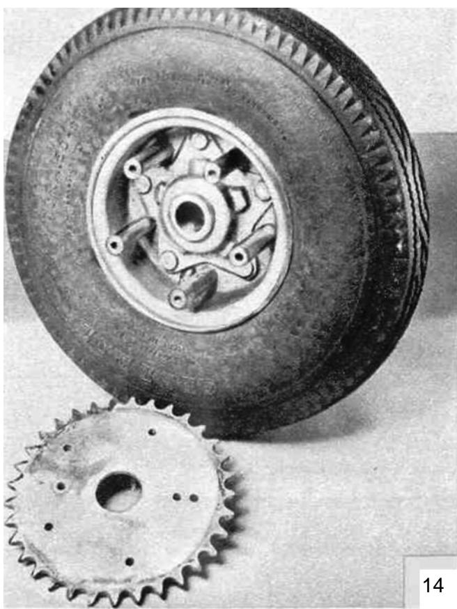
Five spacers, made from standard pipe, are used to keep the sprocket away from hub of the wheel.
