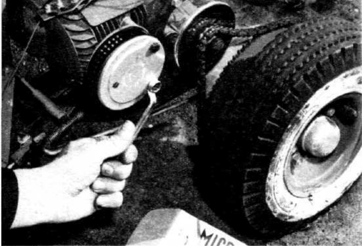
MICRO MUFFLER is shown being bolted over exhaust port of Clinton E-65 engine.
