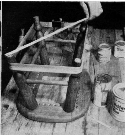
**5** Trestle is square when diagonal measurements are equal. (Note that caning holes are drilled before final assembly.) With glue dry, a disk sander finishes feet to the proper length and angle.
