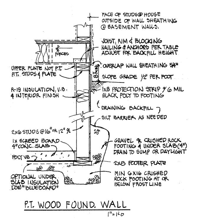
This is a Cross Section detail of the Pressure Treated Wood Foundation wall. You can copy and paste these details onto a plan sheet with your customized basement floor plan.
