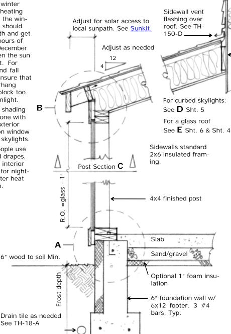
2x6 ledger to standard house wall. Use 2 ledgerlok screws or = to each stud. Provide 1" airflow o/ insulation to sidewall vent.
