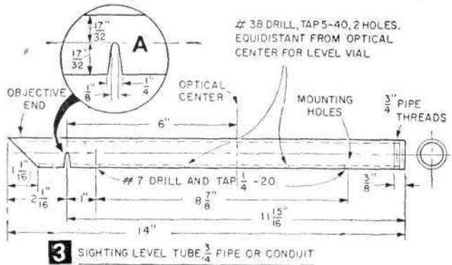
**3** SIGHTING LEVEL TUBE, 3/4" PIPE OR CONDUIT
