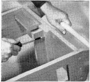
Shaker holder and preassembled rear legs are fastened to the back frame. Drawing at right shows how.
