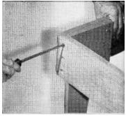
Begin assembly of the unit by securing the front tegs to the side frames with roundhead screws.
