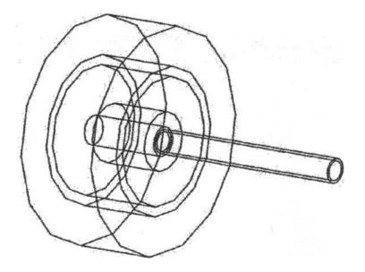
To finish, insert the pipe OR square tube 11" into each end of the rear cross receiver and drill a 1/2" hole completely through the receiver and pipe OR square tube at a centerline point that is 3" back from each end. Insert a  $1/2 \times 6$ " hitch-pin to lock tires into place.
