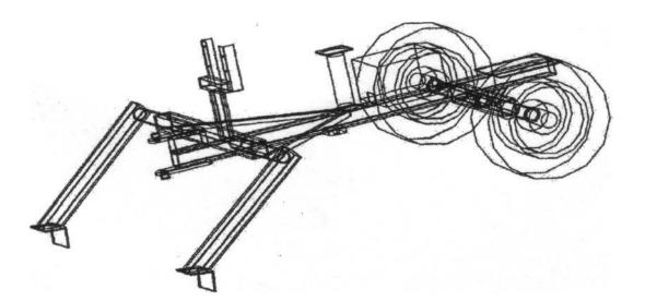
The final step to complete the frame is to weld on the tank and motor mount
