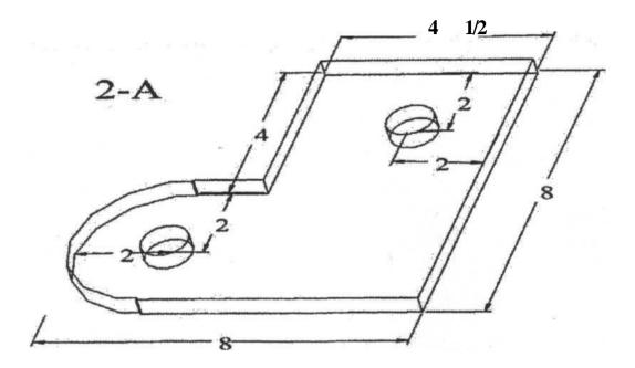
The two pieces are welded to a piece of 3/8" plate that is 8" x 4-1/2". Keep the two pieces parallel to each other. It may help to use two sections of 1" rod (you will need two, 6-1/2" long for this later) placed through both holes to keep them parallel.
