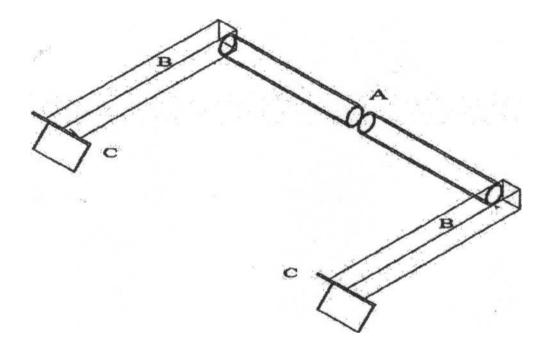
Insert the arms into the front receiver ends so that 11" of the tube is inside the receiver and 11" of the tube is outside. Support the frame on each end so that it is plumb and level. Adjust the height until the outriggers are positioned forward at an approximate 60 degree angle from the frame.
