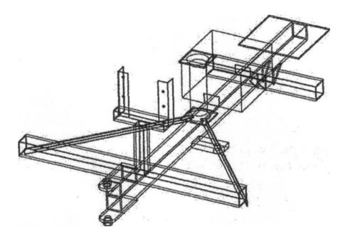
If you are going to tow this backhoe, weld a weld-on 7/8" trailer hitch onto a 36" length of 2-1/2" OD pipe or 2-1/2" x 2-1/2" x 3/16" square tube and insert 12" into the rear of the frame. Drill a 1/2" hole through the frame and pipe or square tube. Insert a 1/2" x 6" pin to lock it into place.
