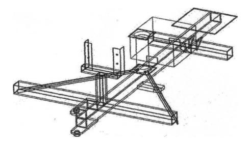
A-2 sections of 2-1/2"OD Schedule 80 pipe, 22" long B-2 sections of 3" x 3" x 1/4" square tube, 30" long C-2 sections of 4" x 4" x 1/4"" angle iron, 7" long
