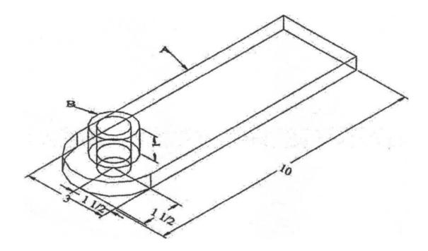
The plates are welded to the front of the frame. Weld the top one on first so that the rear of the plate is flush with the rear of the short piece of square tubing and the plate's mechanical tubing is pointing upward. *See next diagram.*
