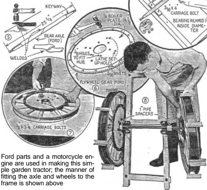
Ford parts and a motorcycle engine are used in making this simple garden tractor; the manner of fitting the axle and wheels to the frame is shown above
