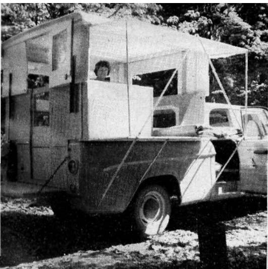
Set up for the night by opening out the side bunk and roof panels and bracing them with conduit. Lower braces rest on hooks that are bolted to truck.
