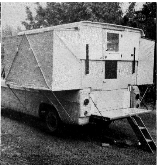
Enclose the camper by attaching plastic or canvas curtains around side bunks. Snap buttons hold them securely. Windows open to provide ventilation.
