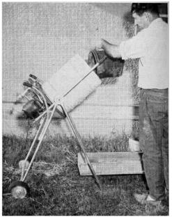
**Loading up.** Mixer takes about a tenth of a bag of cement for most sand-and-aggregate mixes. In final assembly, the frame is sprung apart just enough to admit the trunnions into the supporting washers. Cotter pins prevent trunnions from slipping out and keep frame from spreading while mixer is moved about.
