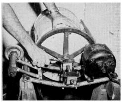
Maple bearings, soaked in oil and dusted with graphite, support drum shaft. Steel straps and J bolts secure bearings. With motor, drum and all parts in place, yoke is balanced to locate trunnions. These are welded 4" forward of balance point so drum swings up.
