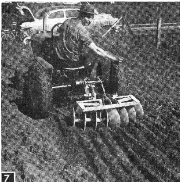
Thorough disking breaks up the clods so small rootlets can get a start. Note the straightened lifting handle. Pulling it forward lifts the implement (plow or disk) when turning at the end of the row.
