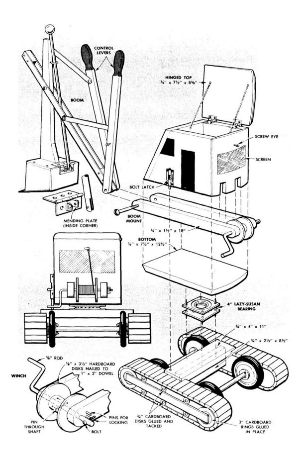
be cut from tin cans or from polyethylene-plastic food containers. Wooden side plates, projecting over the drive wheels and fitting between the bearing wheels, are nailed on.
