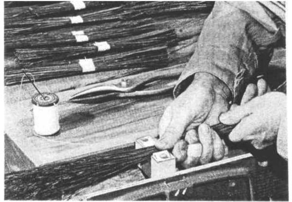
Broomstraws are bundled in a jig, then taped and sewed. Keep the bundles as uniform as possible
