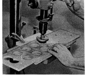
The hole saw is perfect for making the cutouts in the upper half of your Mancala board. If you don't have one, use a jigsaw for this job. To cut out scoring bins with a hole saw, make two overlapping hole cuts and trim the waste to leave a smooth side
