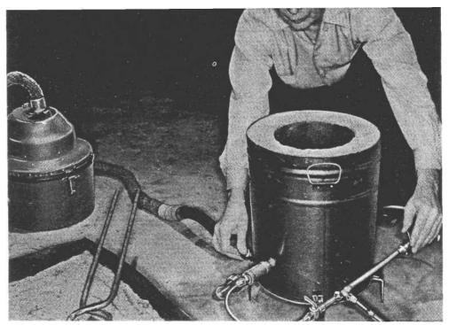
Here's the completed furnace set up ready for use. The burners have separate gas valves to provide precise adjustment of the flame. A single valve controls the air supply from the vacuum cleaner. Although not pictured, the molding flask should be placed near the furnace
