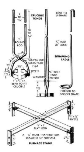
entirely with a piece of asbestos-cement board to retain heat. To inspect the charge you remove the cover with a pair of tongs and observe the contents of the crucible through colored glasses. Use the skimming ladle to drop some borax into the molten metal. Use technical grade borax available at photo-supply houses. Skim off the resulting dross or scum before removing the crucible for pouring.
