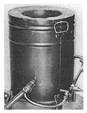
If the rubber hose for the gas line is too small to fit on 3/8-in. tubing, make an adaptor from short lengths of tubing, one fitting inside the other, then sweat-solder together. Also make an adaptor of close-grained hardwood to fit into the end of the vacuum-cleaner hose. Pipe-joint compound is used only at the tees where the half union and reducer screws into the tees, and where the 3/8-in. burner nipples screw into the reducers. All the joints of the gas line should be tested.
