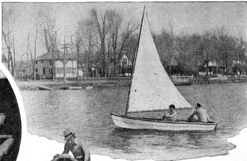
While primarily a rowboat, this stanch little craft can be rigged for sailing. There is a mast step forward, a small centerboard, and a rudder
