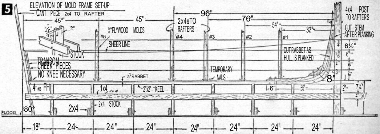
**5** ELEVATION OF MOLD FRAME SET-UP
