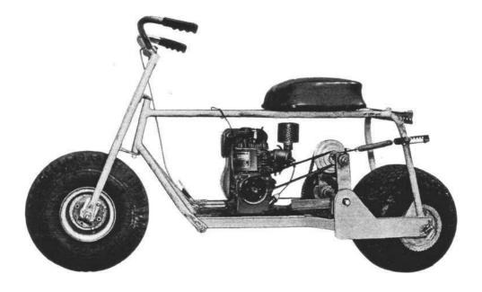
(for light weight) there's no reason why you couldn't use common 3/4-in. pipe or rigid conduit. Also, to avoid the bending, you could join straight lengths with angle iron. Such joints should, however, be reinforced with gussets, since the frame must stand up to severe stresses from jolting over rough ground. You'll also need formed channel for the frame base and transmission rack and steel plate for the engine deck. It's best if axles aren't threaded at the ends, since
