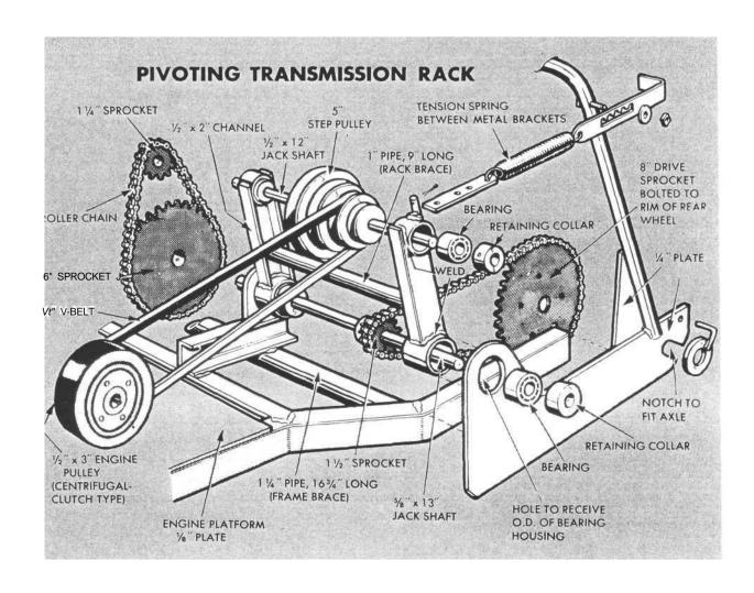
there's too much chance of their being "peened" by scraping past stones. Rather, they should be retained with cotter pins and washers. Special pivoting retainers can be made by welding an L-shape of 1/4-in. rod to one face of a washer large enough to slip onto the axle you've chosen. The tail of the L enters a hole in the plate, holding the axle in place in the notch. (The hub nut shown on the front axle is an alternate treatment.)
