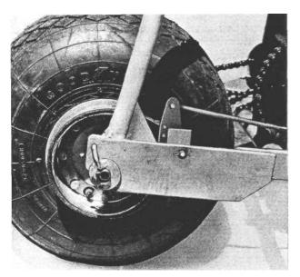
The brake lever is pivoted on top of the rear wheel's hub plate, with a bearing plate between for clearance. The band passes around a drum bolted to the wheel rim. The ends are looped over a pin protruding from the lever's rear face
