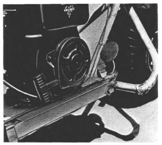
The brake rod passes forward from the lever to the brake pedal at the right stirrup. Note how the pedal angles inward for maximum foot room—and to avoid snagging on underbrush. The fork permits rod adjustment
