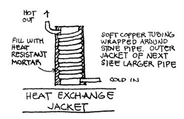
Here is a schematic layout for a wood and solar combination hot water system. You can use one or both as a preheater of water headed to a standard water heater tank. Make sure your tank is installed correctly with working temperature and pressure relief valves — the wood loop can boil water.
