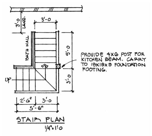
A number of people are in areas where the new IRC building code is in force. Here is a stair that meets that code. The winder at the landing must have a 10" wide tread at 12" in from the corner point. The other treads must also be 10" wide and the risers no more than 7-3/4" tall.
