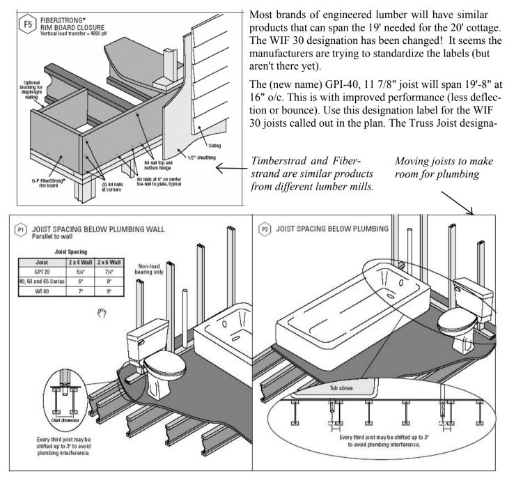
tion for the same span and deflection rating would be a 11 7/8" TJI/Pro-250 @ 16" o/c (spans 19'-5").
