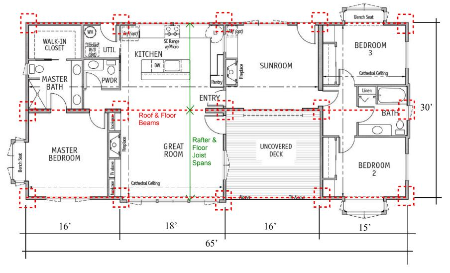
House consists of 4 joined shed roofed modules. The red squares represent the foundation piers. The red line is a beam line under the floor joists and supporting the roof rafters. The floor joists span 15' and should be 2x10 @ 16' o/c. The roof rafters span the same direction (top to bottom) and the same distance. Use 2x10 as well or 2x12 for heavy snow and better insulation. Beams supporting floors and roof have not been calculated.
